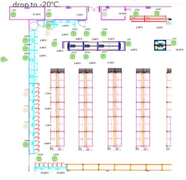
The optimization involved adjusting the demand of the services (refrigeration units), resulting in the compressors maintaining stable consumption within a working band that does not exceed 60% of the total capacity.
