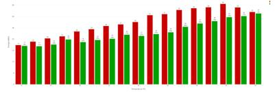
In the graph, we observe the energy consumption of the entire plant at different temperatures, with pre-optimizer data in **red** and post-optimizer data in **green**. We can see that across the entire temperature range, we achieve considerable savings levels.
